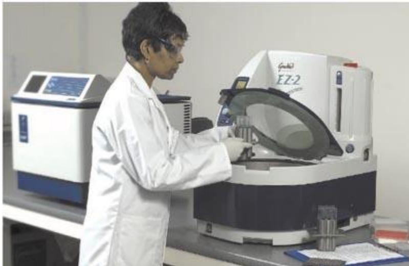
The recent introduction of an EZ2 centrifugal evaporation system for clinical biochemistry sample preparation has provided this particular hospital's laboratory staff with considerable advantages compared with the manual dry down evaporation methods previously used.
